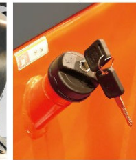
Locked fuel tank cover
