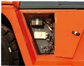
Independent integrated electric cabinet
